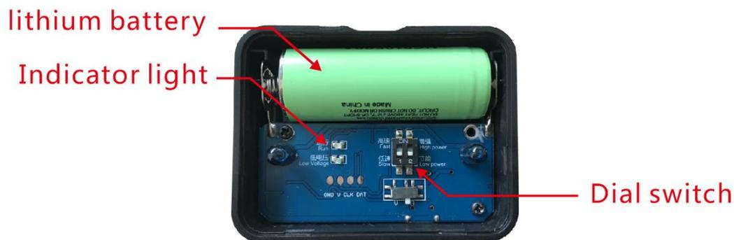
When battery voltage is too low, the red indicator will be flickering to remind you charge or replace the battery. Now we put the infrared transmitter and the passenger flow counting terminal within a face to face position, then the red indicator in terminal stops flickering. This means the device is ready for use.
