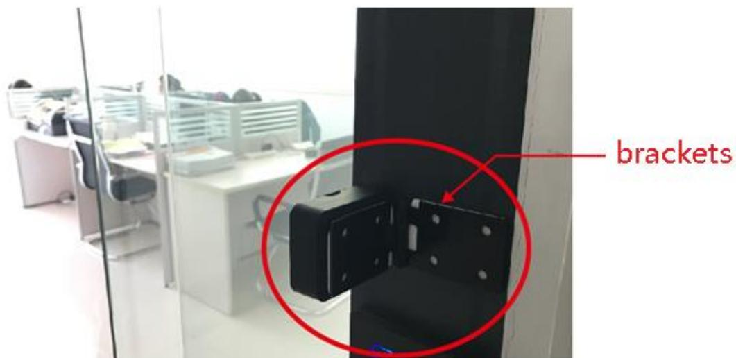
6、 Paste the terminal and bracket by provided double faced adhesive tape, set up the height as about 1.3 meter or equal to local people's average chest height. The terminal already marked an arrow direction which is compliance with pedestrian's actual entering direction. Paste the brackets to installation position and then adjust the bracket angle, using the provided small wrench to fasten the bracket rotary screw. Note, the USB charging port must downwards.
