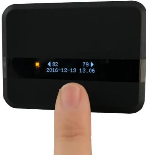
8、 Now let us conduct the parameter setting of terminal, touching this position by hand could awaken screen. Switch to “Keep press to AP”, long press till screen displaying “AP start”. Open smartphone’s WLAN, we can see a iDTK network, connect to this network, OK, now we have successfully connected to iDTK network.
