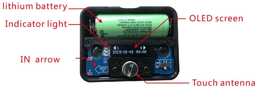
This is touch antenna, when we are conducting touch operation, the yellow indicator light will light up. We can inquiry various information the counting terminal through touching operation, such as current power, product ID, working parameters and working period. Such information is automatically downloaded by this counting terminal from cloud or set up by phone.
